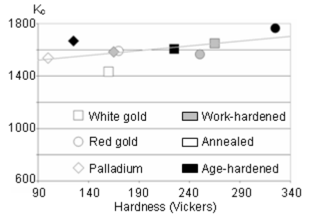
Figure 11: Correlation between hardness and specific energy (measured in identical working conditions) in case of milling.
